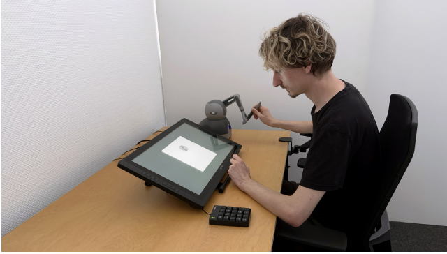
Figure 2: A participant interacts with a stimulus using a desktop display and a force-feedback device during a trial.
